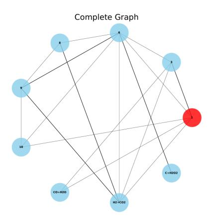
$graph\_kin.pdf$  is a graph displaying only those nodes actively participating in the kinetics at the chosen temperature T or energy E. Here, the widths of the edges are proportional to the total (forward + backward) flux in the kinetics simulations. The starting node is shown in red.
