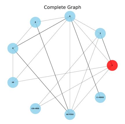
$graph_kin.pdf$  is a graph displaying only those nodes actively participating in the kinetics at the chosen temperature T or energy E. Here, the widths of the edges are proportional to the total (forward + backward) flux in the kinetics simulations. The starting node is shown in red.
